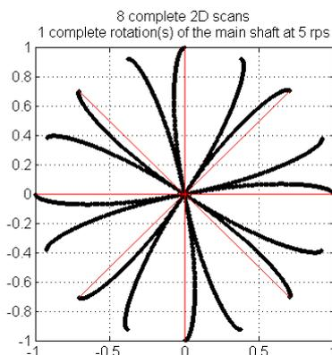
Fig. 4 Sample of trajectory drawn by the director vector on a plane perpendicular to the external axis and located 1 m ahead of the scanner mirror. Case when the 2D scan is at 40 Hz and the external shaft speed is 5 rps.
