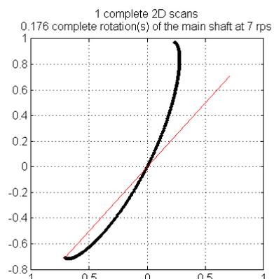
Fig. 7 Sample single scan drawn by the projection of the director vector. Case when the 2D scan is at 40 Hz and the external shaft speed is 7 rps.
