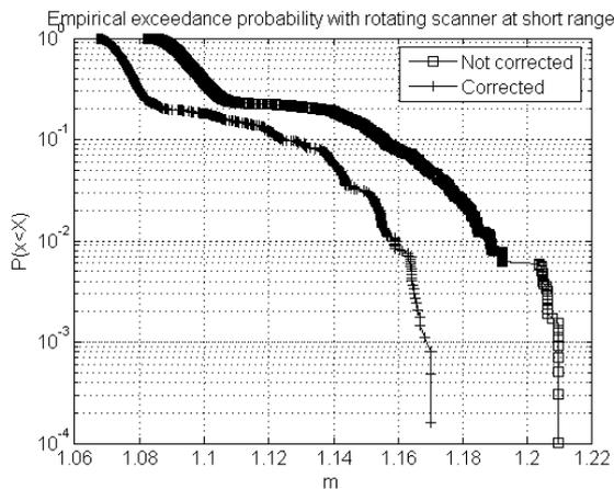
Fig. 11 Empirical exceedance distribution for short range, for real data collected when rotating the scanner.
