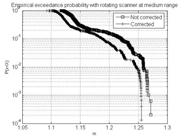
Fig. 12 Empirical exceedance distribution of distance for medium range, for real data collected when rotating the scanner.
