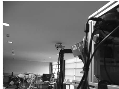
Fig. 9 Experimental setup with leveled range finder scanning the ceiling.
