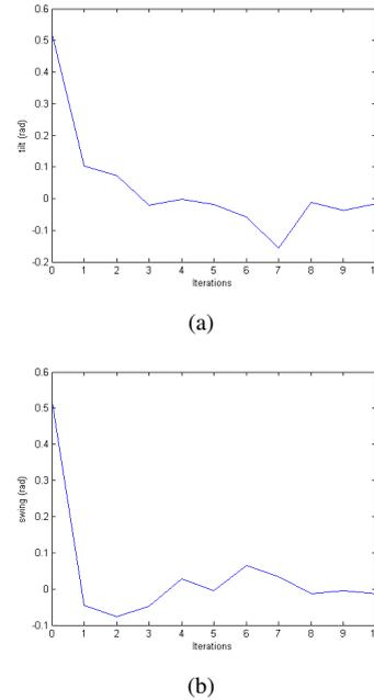
Fig. 2. Evolution of the tilt (top) and swing (bottom) angles along the iterations of the Broyden's method. Initial configuration:  $\theta_{tilt} = \frac{\pi}{6}$   $\theta_{swing} = \frac{\pi}{6}$
