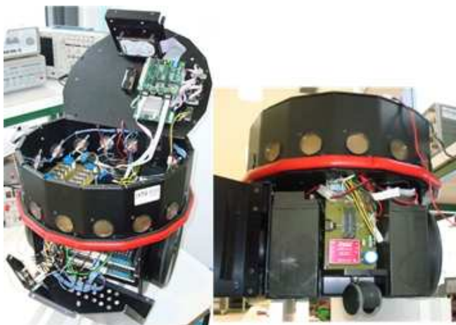
Fig. 1. The New Scout. In the left image, the SuperScout's top and bottom lid are open, revealing its new interior hardware. On the right the posterior battery bay is also open, showing the circuit-board dedicated to power distribution sided by the two 12Volt batteries.
