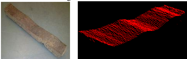
Fig. 8 Real cork piece (left). 3D reconstruction (right).
