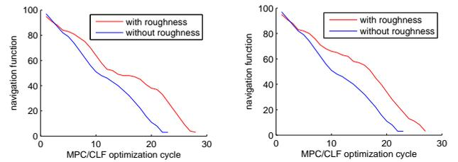
Fig. 7. Value of navigation function at the end of optimization cycle along the selected path
