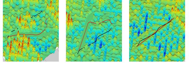
(a) Case I: Flat section of terrain appearing on the right hand side (b) Case II: Flat section of terrain appearing on the left hand side (c) Case III: Narrow flat section of terrain appearing in the front side
